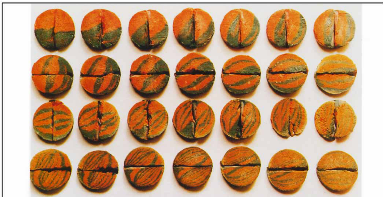
Figure 5. Successive slices of the mixture along the first four blades.
